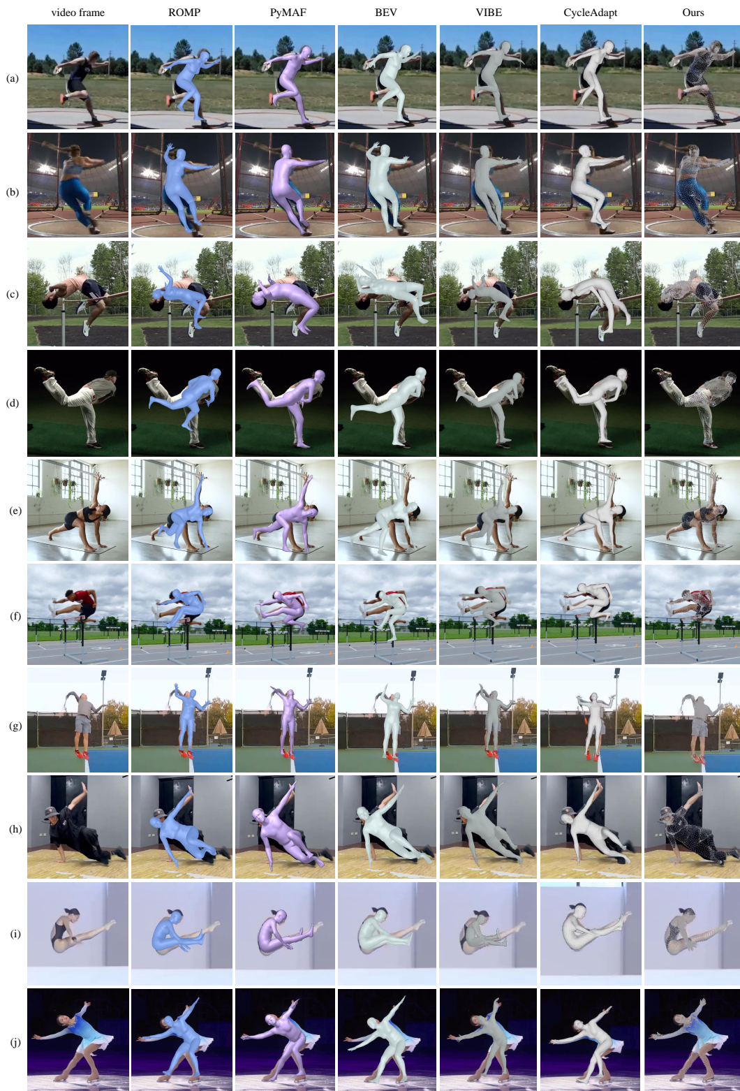
Figure 10: Qualitative comparisons of 3D pose reconstruction results between ROMP [32], PyMAF [41], BEV [33], VIBE [24], CycleAdapt [28], and ours.
